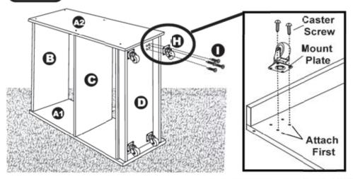
With the unit still on its side, attach 4 Wheel Casters(H) into the holes underneath Bottom Shelf(D) using 16 Caster Screws(I), using 4 in each. Start with the 2 centermost holes as shown below. Tighten with a Phillips Head Screwdriver.
