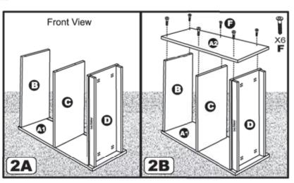
2B. Position Right Side(A2) to all the screw holes line up with all the holes in the 3 Shelves(B,C,D). Secure Right Side(A2) to the assembled unit using 6 Hex Head Screws(F). Tighten with the Hex Key Tool(G).
