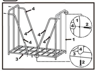
Attach the 4 Braces(4) to the Side Panels(1) and Base(3) using 8 Screws(2) as shown. Tighten with the Allen Wrench(7).
