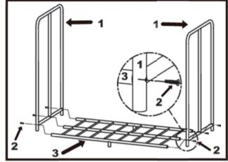
Attach the 2 Side Panels(1) to the Base(3) using 6 Screws(2).
