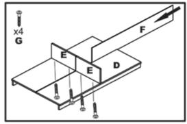
1A. Secure the 2 Lower Dividers(E) to Bottom Shelf(D) using 4 Hex Head Screws(G), using 2 in each. Tighten with the Hex Key Tool(H).
