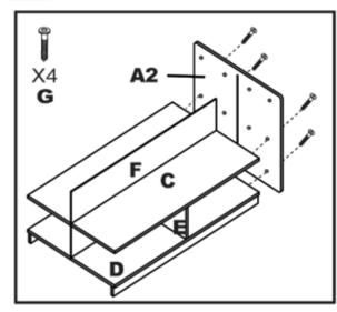
2A. Position Right Side Panel(A2), so the 4 pre-installed wooden dowels in the ends of the shelves are fully inserted into the holes located inside Right Side(A2).
