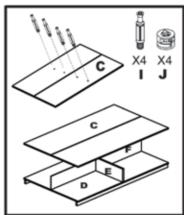
Insert 4 Metal Dowels(I) into the plastic plugs located underneath Center Shelf(C).
