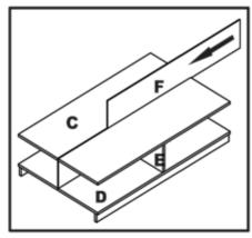
1F. Slide Divider(F) into the slot in the top of Middle Shelf(C) until fully inserted as shown.
